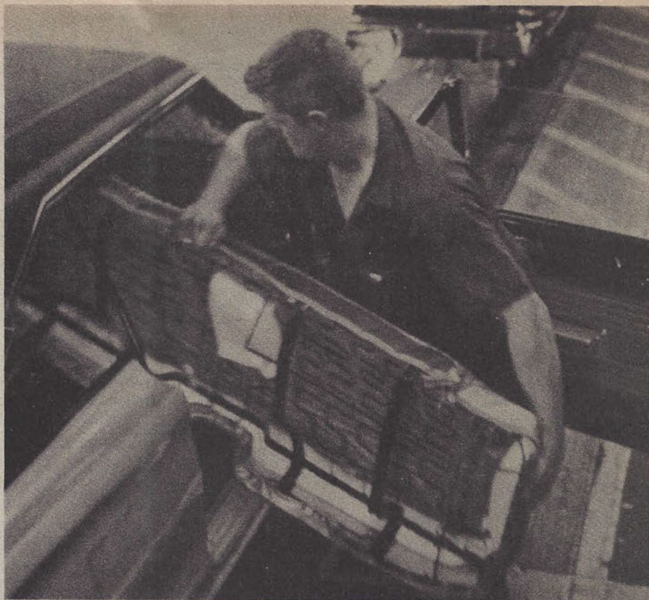
This workers has one minute in which to insert the back seat of a car.
